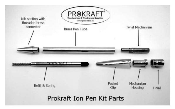
1] Drill your blank using Atom2 drill, abrade the surface of the brass pen tube lightly and glue inside the blank using your preferred adhesive. The drill flutes are slightly shorter than the blank length so ensure you withdraw the drill regularly to remove swarf and allow the drill to cool if necessary. This process is commonly known as pecking – it is very important especially for acrylic blanks to prevent overheating / melting.
